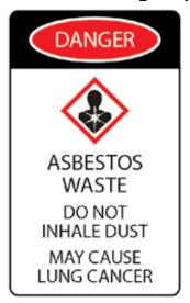
**B:** Sample Asbestos Removal site signage
